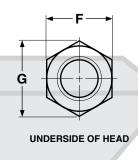
‡Length of a cap screw is measured from the underhead bearing surface to the extreme end of the screw.
